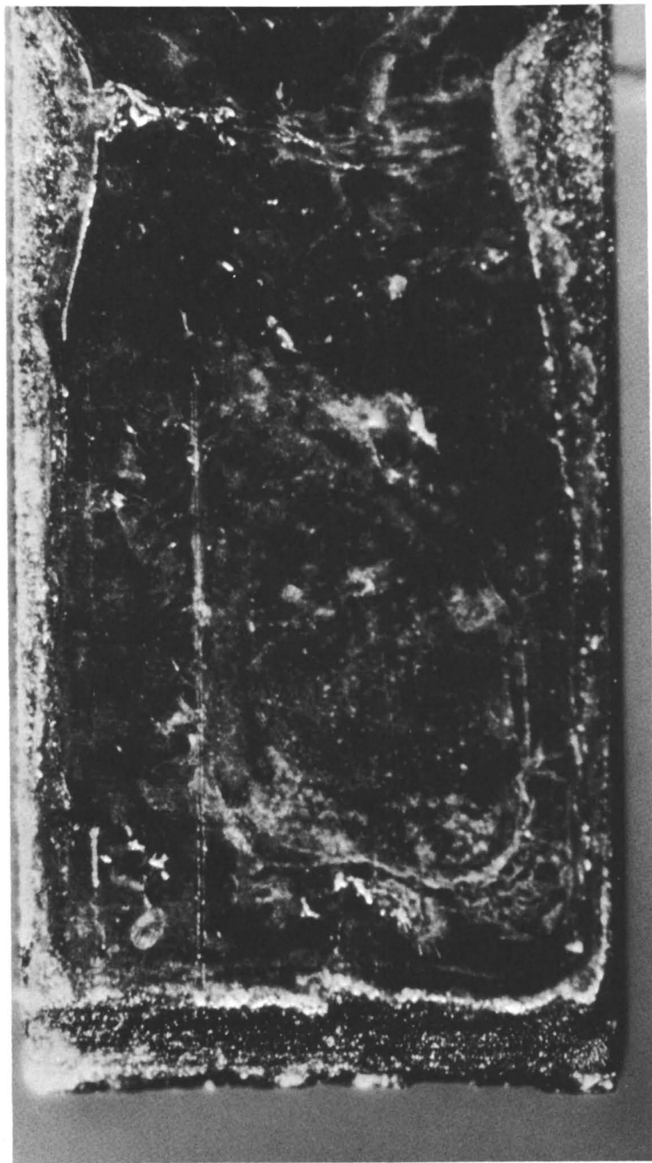
Figure 14. Photomicrograph of a poorly plated tooth of a circuit board connector.
