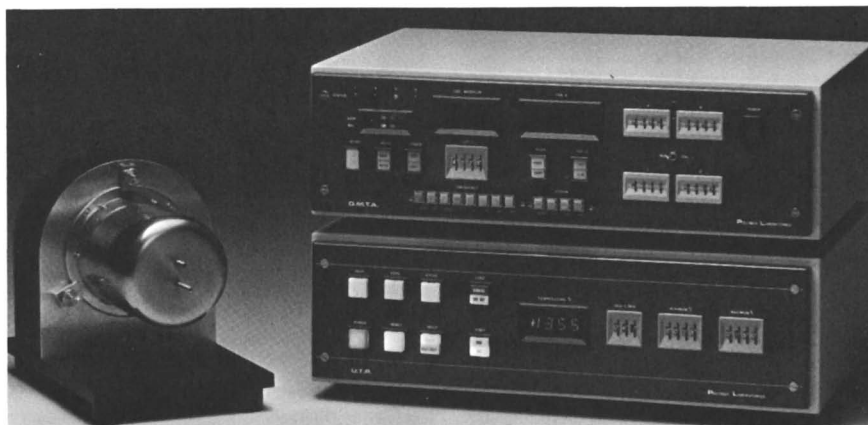
Figure 1. The PL-dynamic mechanical thermal analyzer. Key: the mechanical measuring head, left; the dynamic analyzer unit, top right; and the temperature programmer, bottom right.
