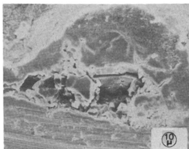
Figure 11. Cross-section of aluminum siding defect (350 \times ).
